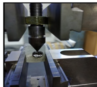
Figure 4. Application of oblique cyclic loading on the specimens
