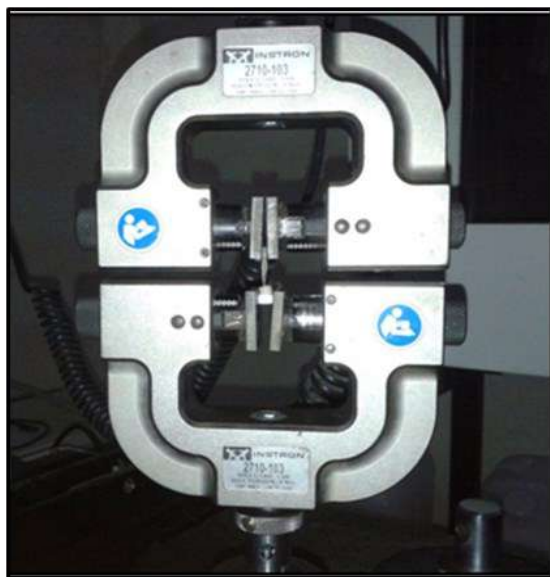
Figure 7. Evaluation of Micro-tensile bond strength at core ceramic and layered ceramic.
