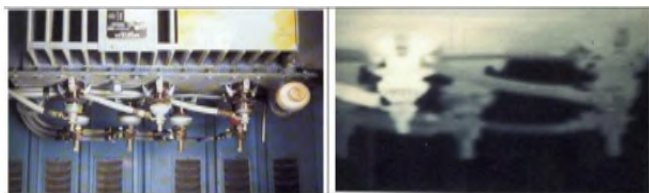
Figure 1. Visible Image (Left) and infrared (right) of a transformer of electrical connection.
